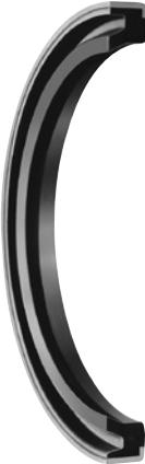
The profile AF Ultrathan® wiper ring serves the purpose of preventing the penetration of dust, dirt, sand, and metal swarf into hydraulic cylinders. This reduces the risk of scoring caused by contaminants from external sources imbedded in the sliding parts. The excellent wiping effect is achieved by the special design of the wiper lip.
