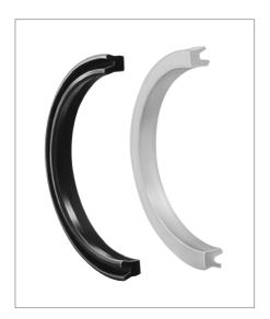
The Ultrathan® sealing set profile KS has been developed especially for sealing pistons in dual media hydraulic accumulators. The shape of the seals makes them ideal for the permanent separation of the pressurized media e.g. oil and gas with low friction forces.
